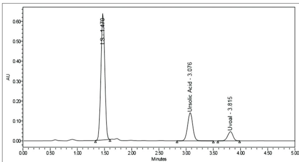
Fig 2. UPLC analysis of a sample containing 100  $\mu$ g/mL of ursolic acid and uvaol as well as 20 $\mu$ g/ml of the internal standard
