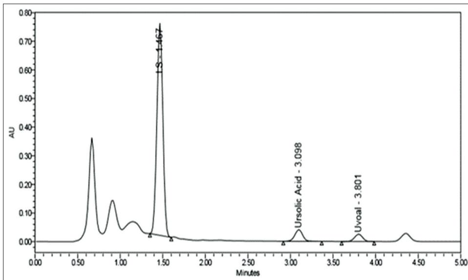
Fig 6. Determination of ursolic acid and uvaol in dry oregano (planted in Spain) in the presence of internal standard.
