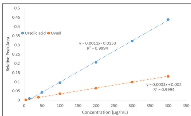
Fig 3. Calibration curve for ursolic acid and uvaol
