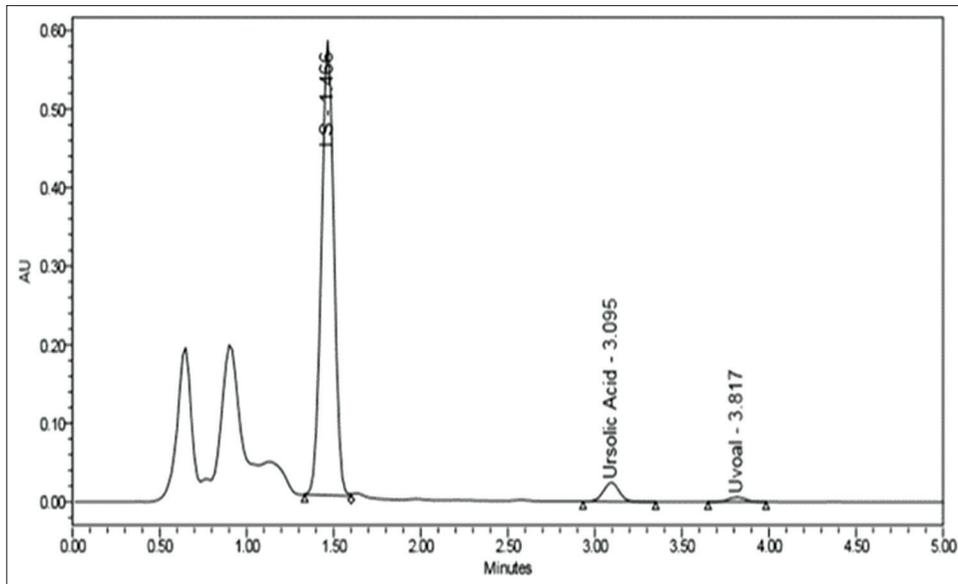
Fig 5. Determination of ursolic acid and uvaol in dry oregano (planted in Palestine) in the presence of internal standard.
