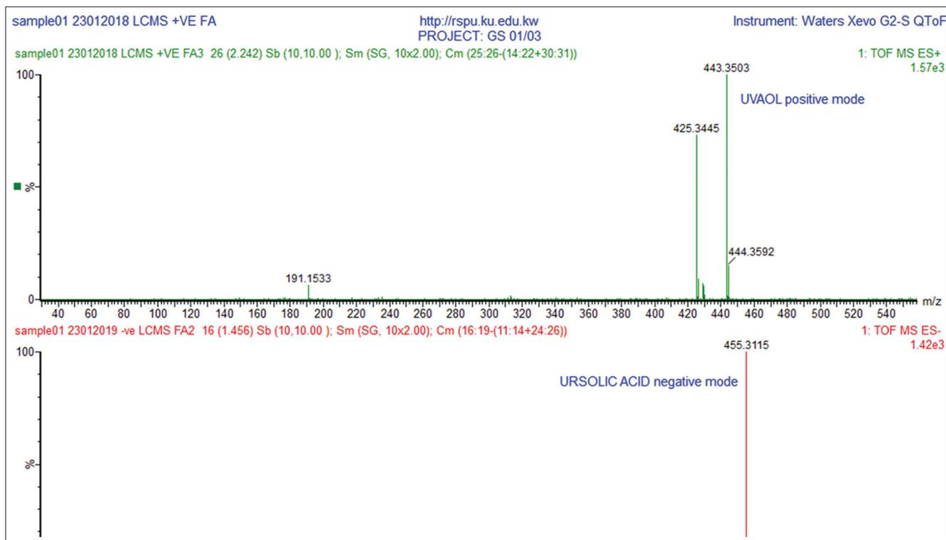
Fig 7. MS Spectra of ursolic acid (negative mode) and uvaol (positive mode) performed on mass spectrometry.
