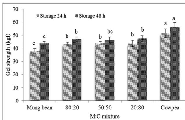
**Fig 2.** Gel strength of mung bean (M) and cowpea (C) starch at different ratios. Results are mean±standard deviation of triplicate determinations. Mean values of different letters a, b, c in the same bar graphs are significantly different ( $P < 0.05$ ).
