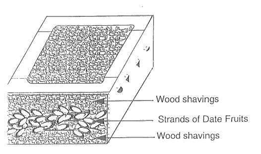
Fig 1. The developed system to prolong the uptake of treatment solution and to reduce air movement around fruits during cold storage of date. Note that date strands are embedded between two layers of small pieces of wood shavings.
