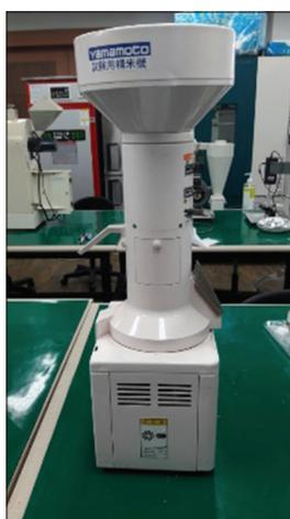
Fig 5. Friction type miller.
