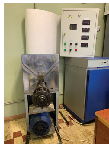
Fig 2. Device for cold pressing MPL-1.
