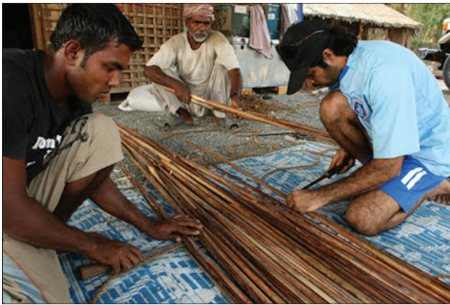
Fig 4. Fujairah, UAE. Assembling date leaf midribs for the base of a shasha. Source: Pound 2009.
