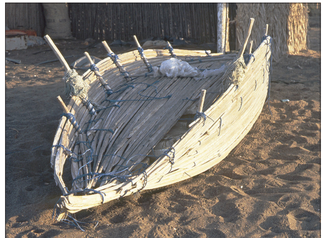
Fig 6. A Larger shasha date leaf fishing boat, Batinah Coast, Gulf of Oman. Note that nylon rope is used in the construction. Undated photo. Used with permission of OMAN-FOTOALBUM
