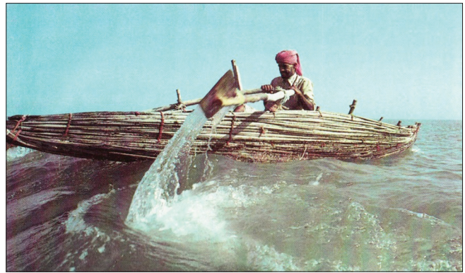
Fig 5. Small one-man shasha date leaf fishing boat at sea off the Batinah Coast, Gulf of Oman, Oman; photo dates to the early 1980s. Note the traditional rope binding together groups of midribs. Source: http://indigenousboats.blogspot.com/2012/04/shasha-arabian-bundle-boat.html
