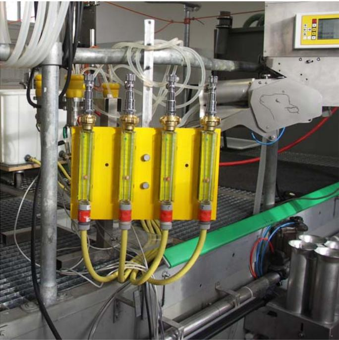
**Figure 2. Overview of the whole test set-up: Flow simulation at the milking system Multilactor® in the laboratory.**
