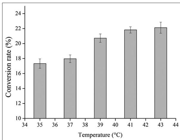
**Fig 2.** The biotransformation was performed in triplicate at temperature range from 35 to 43°C, and the fermented 24 hours with 5% inoculum.
