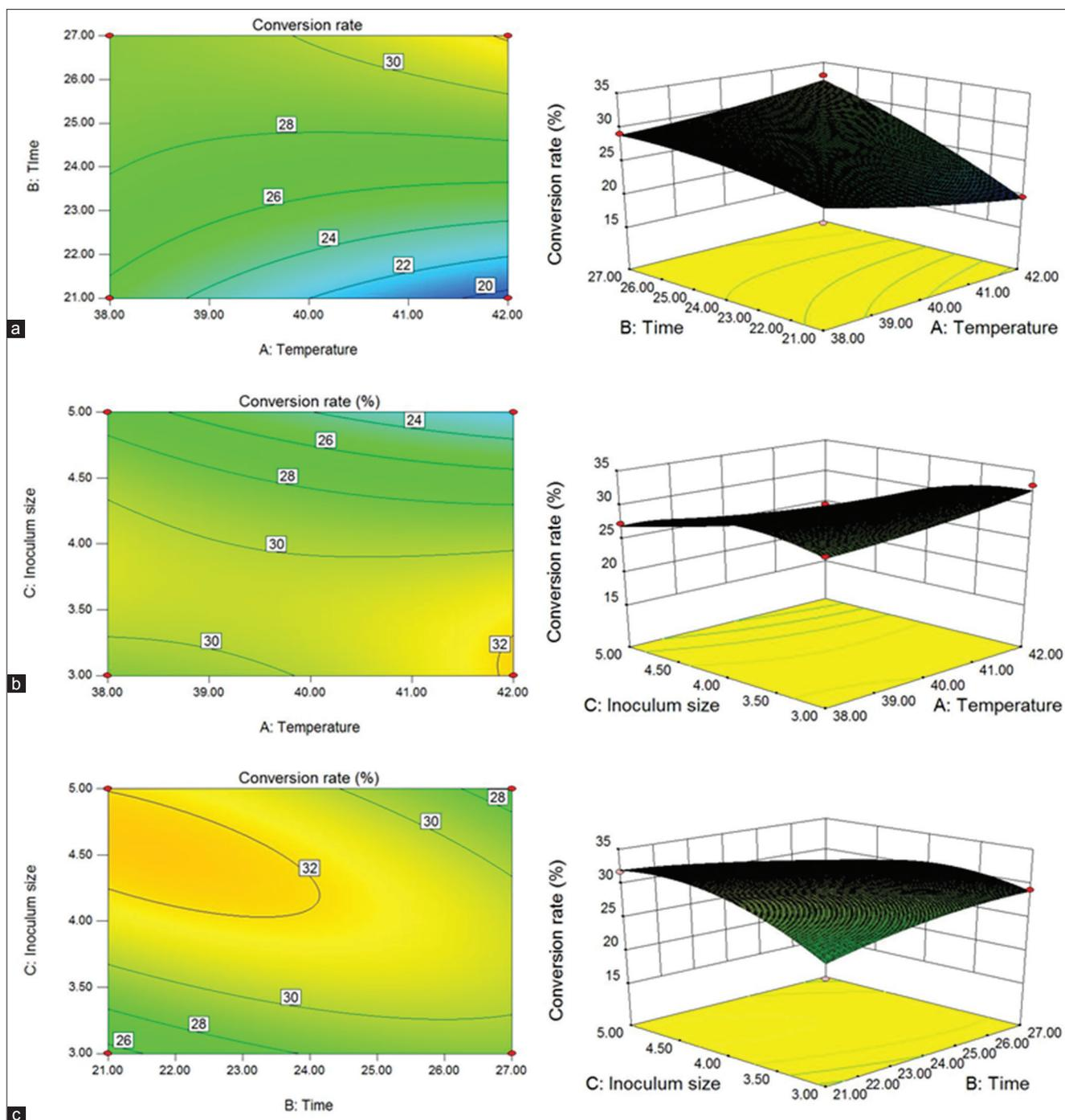
**Fig 5.** Response of conversion rate using the Central composite design obtained by plotting: (a) temperature versus time (inoculum size, 4%); (b) temperature versus inoculum size (24 hours); and (c) time versus inoculum size (43°C).
