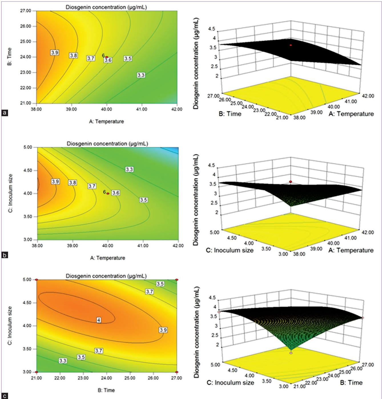
**Fig 6.** Response of concentration of diosgenin using the Central composite design obtained by plotting: (a) temperature versus time (inoculum size, 4%); (b) temperature versus inoculum size (24 hours); and (c) time versus inoculum size (43°C)
